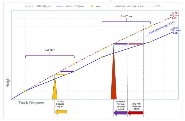
For distance uncurl: In a different fashion; the Error height adjustment is not additive. The error relates only to the obstacle's most recent turn. This is because the most recent turn start location, already entails accurate information of height.
