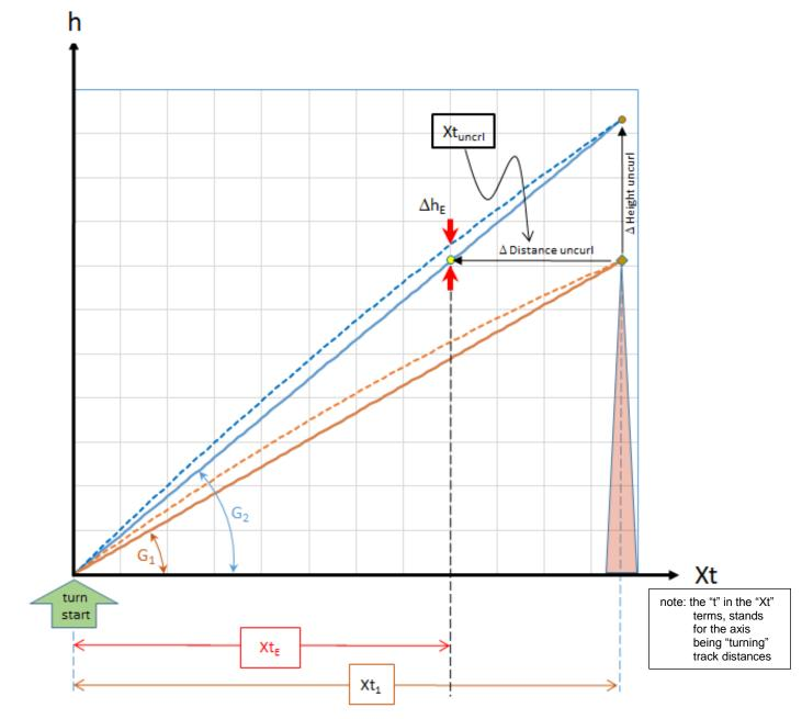
Premise: The Actual Flight Path is to be modeled as a parabola with Equation:  $A (Xt)^2 + B Xt + 0 = h$ (where "A" and "B" are the constants)
