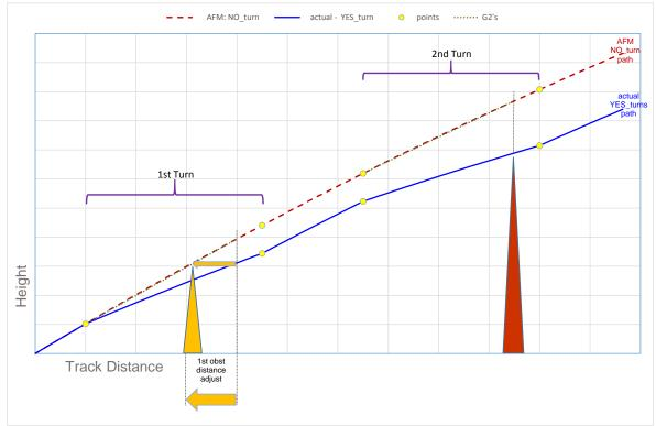
But, for the obstacle in the second turn; if only its 2nd turn height adjustment is applied, it will fall short of reaching the AFM NO\_turn path. The 2nd turn gradient decrement will have been uncurled only to a flight path where the 1st turn gradient decrement still exist.
