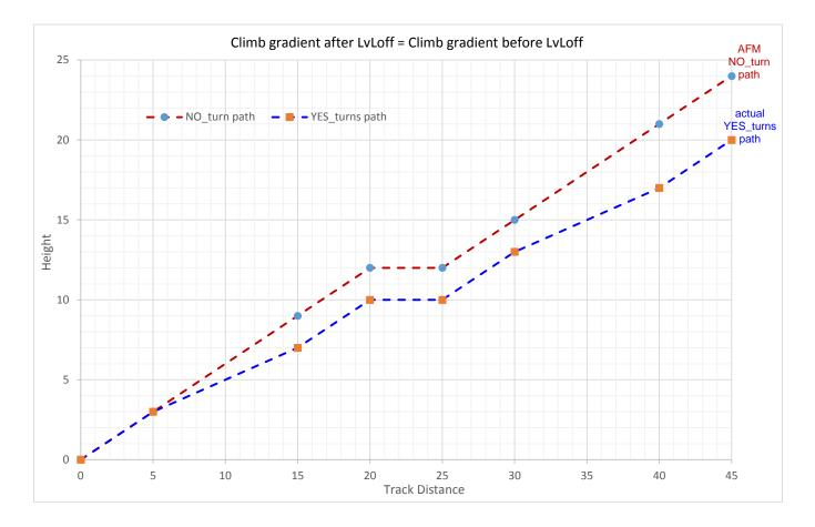
The prior exaggerated scale sample sketch has been built for illustration purposes with an arbitrary 60% climb gradient before and after the turn. Climb gradient after the level-off = climb gradient before the level-off.
