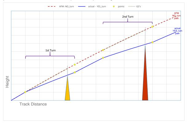
The obstacle in the 1st turn correctly uncurled on the AFM NO\_turn path.
