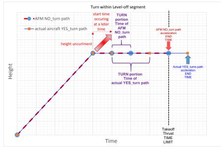
Yet, precisely because it's the AFM calculated path, it can be made to ensure the fulfillment of acceleration within the Takeoff thrust time. The sought after consequence of this, is that: After a height uncurl of the level-off, the <u>AFM NO\_turn path acceleration END **Time** value</u> will be greater than or equal to the <u>YES\_turn acceleration END **Time** value</u>.
