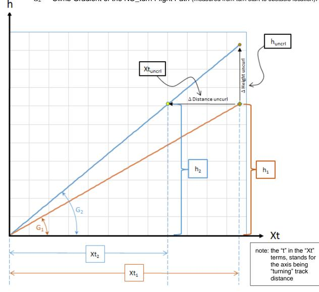
The simplest way to grasp the essence of the above equation is to recognize that the gradient  $G_2$  is the relation of  $\Delta$ Height /  $\Delta$ Distance in the NO\_turn path line. So from any point in the YES\_turn path; a  $\Delta$ Height to the NO\_turn path can be converted to a  $\Delta$ Distance to the NO\_turn path, when dividing it by  $G_2$ . Hence, a  $\Delta$ Height uncurl defined by Xt<sub>1</sub>(GrdDec), when divided by  $G_2$ , becomes a  $\Delta$ Distance uncurl.
