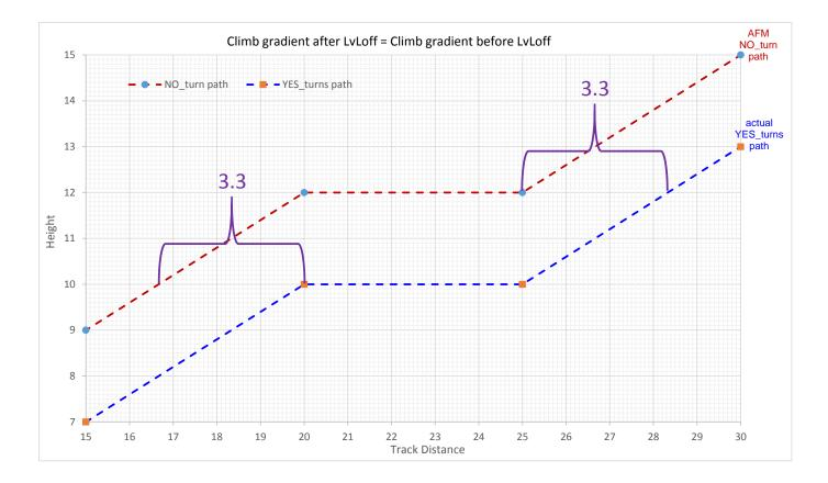
If the climb gradient after the level-off is greater than the climb gradient before the level-off; then, by geometry, the distance displacement after the level-off will result of a lower value than the distance displacement before the level-off.
