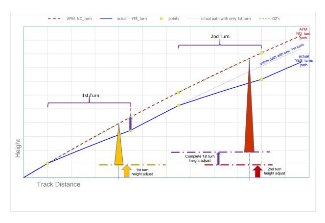
The height uncurl adjustment from preceding <u>complete</u> 1st turn must also be added in order for the obstacle top to be correctly uncurled on the AFM NO\_turn path.
