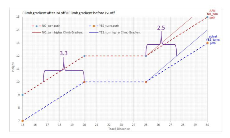
The application of the prior to the level-off, 1st turn's 3.3 distance displacement to the turns after the level off will generate a conservative distance displacement margin to the turns after the level-off. In the above scale sample sketch, the conservative margin = 0.8 distance units (3.3 - 2.5).
