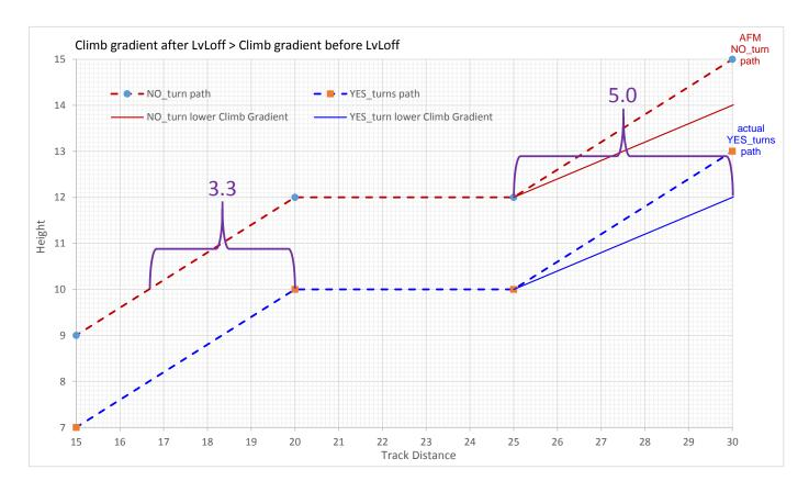
The application of the prior to the level-off, 1st turn's 3.3 distance displacement to the turns after the level off will generate a hampering error to the regulatory compliance displacement of the turns after the level-off. In the above scale sample sketch the hampering error = 1.7 distance units (5.0 - 3.3).
