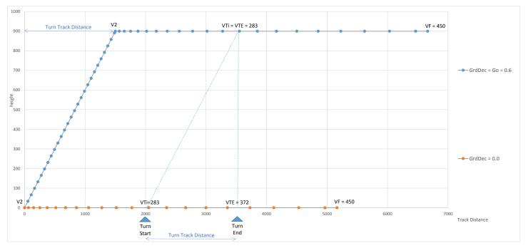
Boundary Case 1: the 2nd Sgmnt Gradient decrement due to Turning = the 2nd Sgmnt Climb Gradient capability. Boundary Case 2: the 2nd Sgmnt Gradient decrement due to Turning = 0.
