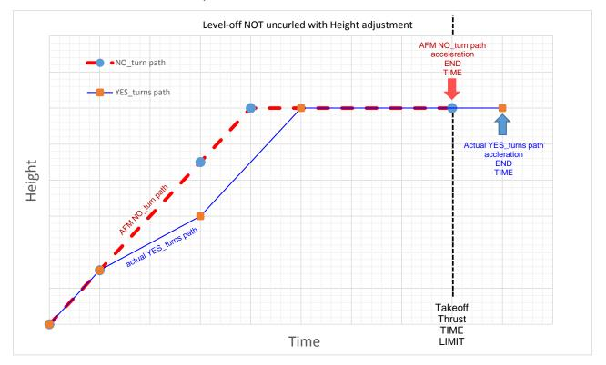
Note that in the above path plotting, the horizontal axis is "Time". Keep in mind that at constant velocities, Time is proportional to Distance. In turn, at constant  $V_2$  airspeed: Time will be reasonably proportional to Distance.
