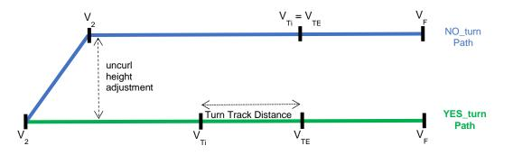
Within accelerating Segment from  $V_2$ -to-VTi : YES\_turn VTi-to-VTE -vs- NO\_turn Clb\_at\_V<sub>2</sub> : Within accelerating Segment from VTE-to-VF : NO\_turn Path Time = Yes\_Turn Path Time NO\_turn Path Time ≥ Yes\_Turn Path Time NO\_turn Path Time = Yes\_Turn Path Time
