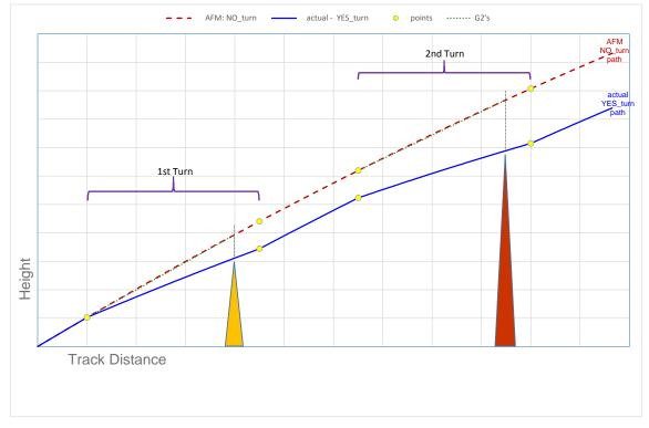
In the sketch below, the obstacle in the 1st turn correctly uncurls on the AFM NO\_turn path. But, for the obstacle in the second turn; if only its 2nd turn height adjustment is applied, it will fall short of reaching the AFM NO\_turn path. The 2nd turn gradient decrement will have been uncurled only to a flight path where the 1st turn gradient decrement still exist.
