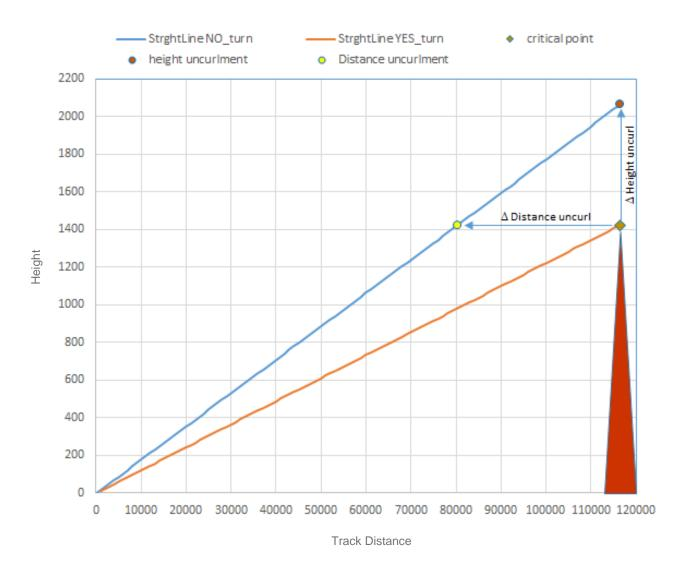
FACT: height uncurl will make the AFM perform obstacle clearance calculations at higher Heights than the aircraft will in reality be flying at, when over the obstacle.
