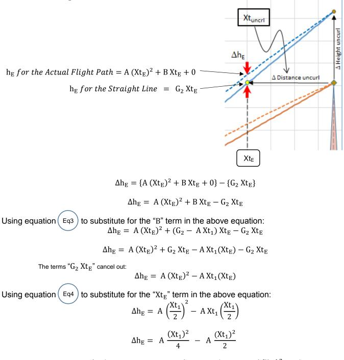
$$\Delta h_{\rm E} = \frac{A}{2} \left( \frac{1}{2} (Xt_1)^2 - (Xt_1)^2 \right) = \frac{A}{2} (Xt_1)^2 \left( \frac{1}{2} - 1 \right) = \frac{A(Xt_1)^2}{2} \left( -\frac{1}{2} \right)$$
