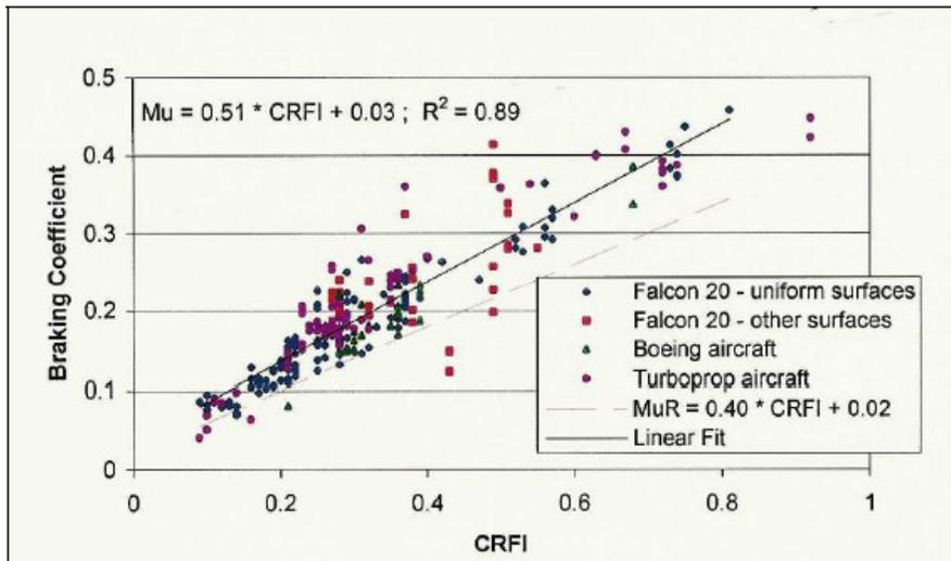
The basic problems were the precision of the friction devices and of variability of runway conditions. The friction measuring devices gave a relatively wide range of readings for the same condition and correlating them to aircraft performance did not yield a tight, linear fit. Not only that, but there were some glaring outliers in the data that resulted from certain contaminants.
