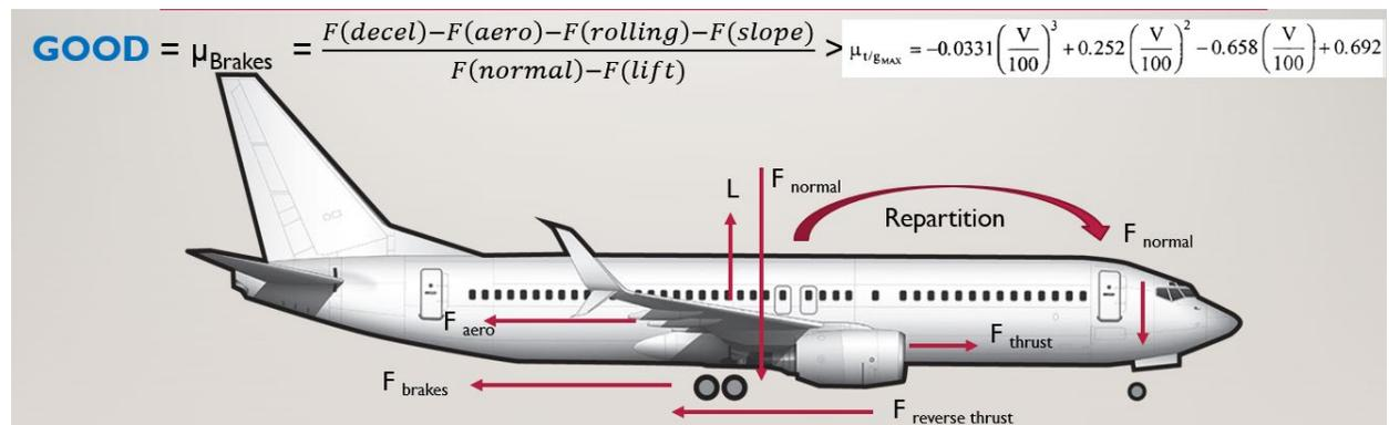
Figure 12 Wheel Brake Coefficient calculation process (Four Winds Aerospace)
